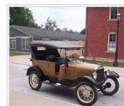
The Ford Model T was the first commercial flex-fuel vehicle. The engine was capable of running on gasoline or ethanol, or a mix of both.
