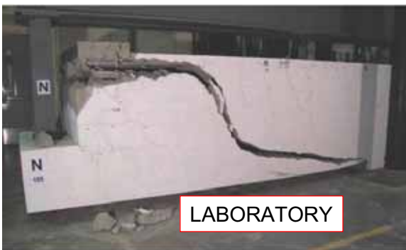
Figure 5.7 Failure of the "as-built" cantilever during the laboratory loading tests at McGill University
