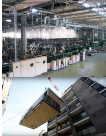
Automatized prefabrication of building modules
